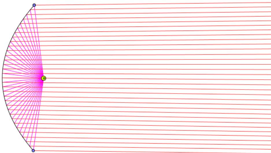
When the source of light is a bit ahead of the focus of a parabola and the source of light is shaded from below we get the low-beam:
