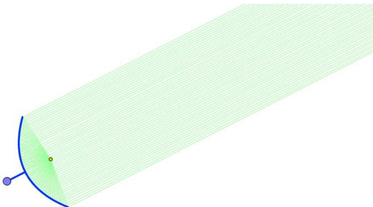
If the satellite dish is not correctly positioned, lots of 'rays' are lost, because they are reflected away from the focus and the sensor. Consequently, the TV reception is poor.
