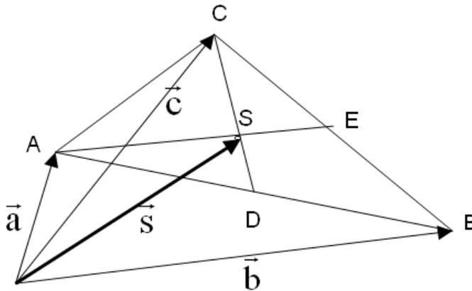
The following reasoning makes use of the fact that the point of gravity S is the medians' point of intersection (here CD and AE) and that the medians are divided by S to a ratio of 1 : 2 and the sections, consequently, are 1/3 respectively 2/3 the length of the medians.
