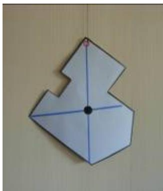
Balancing it with the index finger confirms the position of the centre of gravity.
