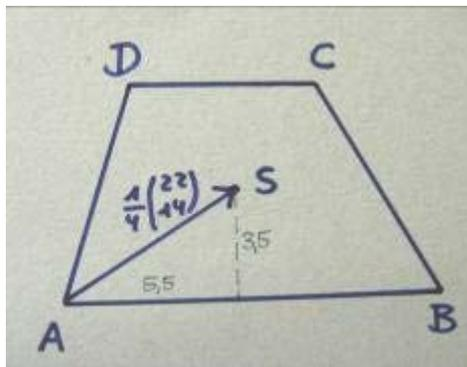
d) The position of the centre of gravity is confirmed (considering experimental inaccuracies) by the suspension method.
