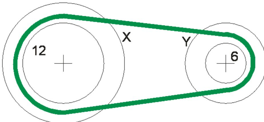
Figure 3: The chain connects the 12-teeth chainring in front with the 6-teeth chainring at the back.
