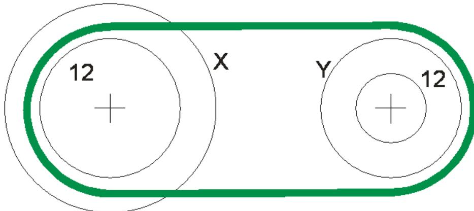
Figure 2: The chain connects the 12-teeth chainrings.
