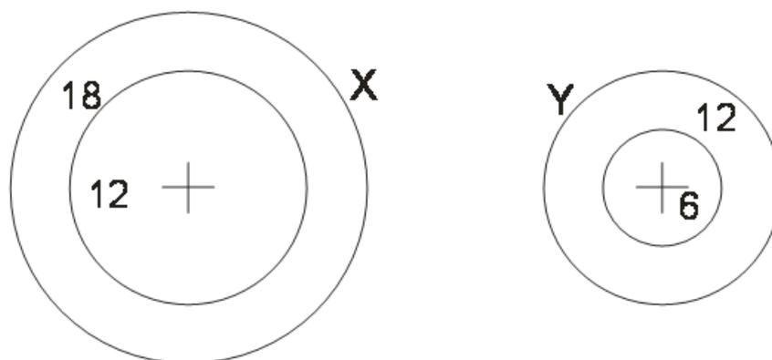
Figure 1: Front chainrings with 18 and 12 teeth and back chainrings with 12 and 6 teeth
